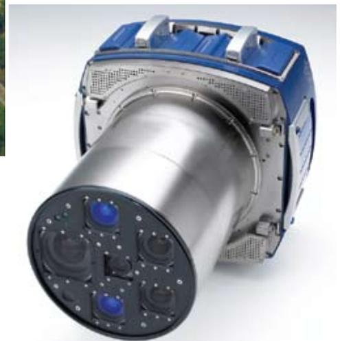
Z/I Imaging DMC II four-band digital sensor
